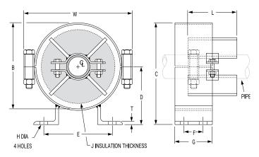
Pipe Alignment Guide: Figure 255, Size C thru J
