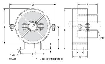
Pipe Alignment Guide: Figure 255, Size A & B
